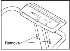
Remove the bolt and washer from the lower end of the upright. Lay the upright on the treadmill. **Keep all bolts and washers in a secure location.**
